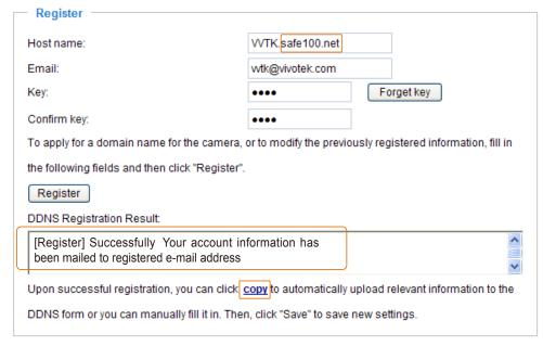
3. Click **Copy** and all the registered information will automatically be uploaded to the corresponding fields in the DDNS column at the top of the page as seen in the picture.
